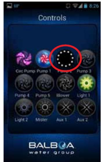
Depending on your coverage and data speed, the response time for acknowledging a device press may vary. You will know the app is waiting by the small spinning dots. If the operation mode of the function is not changed after pressing the button, repeat the operation.
