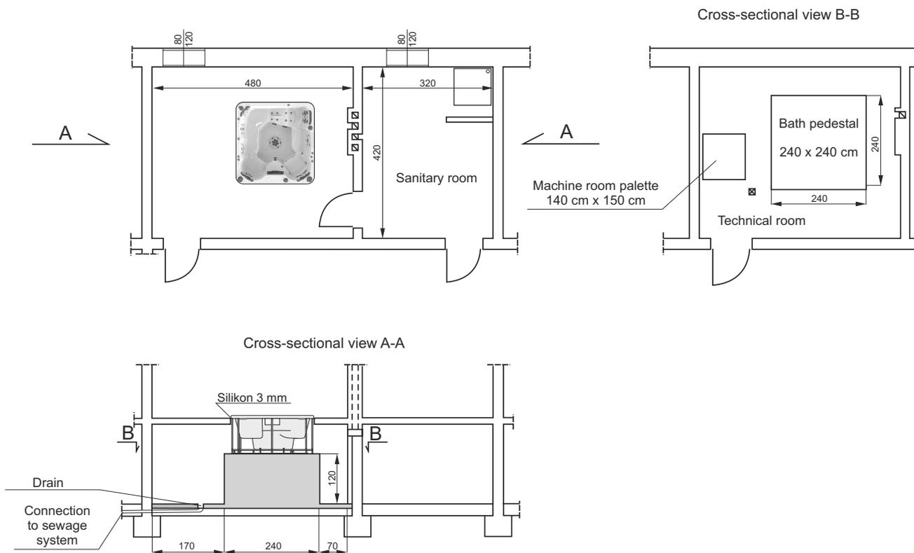
**Bath installed on top of the floor slab**
