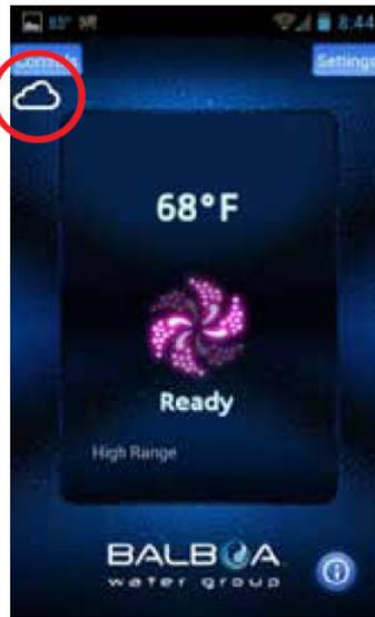
If you are using a Wi-Fi hotspot or cellular data (3G/4G) network to connect to your tub via the Internet you will see a Cloud icon letting you know you are connected remotely.
