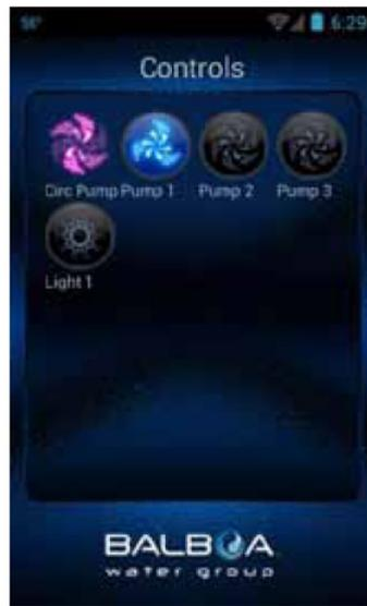
You can now turn on your pumps & lights by pressing the Controls button. The equipment for your tub will automatically show up on this screen. You can turn the devices on/off by pressing the buttons.
