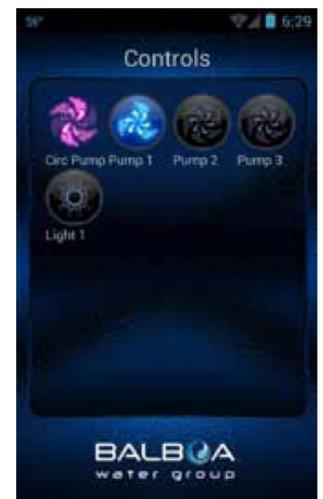
You can now turn on your pumps & lights by pressing the Controls button. On Android™, use the back/return key to return to the main app screen.
