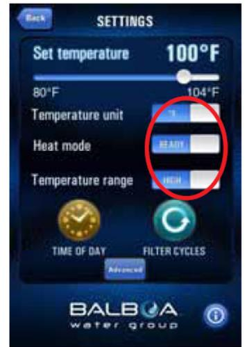
Slide the bar to set the temperature you want the water to heat to. The Set Temperature will adjust accordingly as you move the slider.
