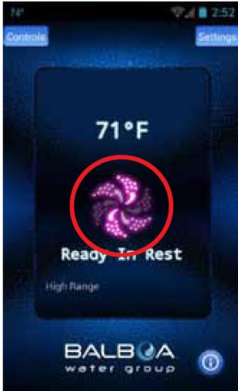
The main pump is on and the heater is on. The icon is red/pink and is moving
