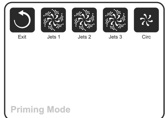
**Important:** A pump should not be allowed to run without priming for more than 2 minutes. Under NO circumstances should a pump be allowed to run without priming beyond the end of the 4-5 minute priming mode. Doing so may cause damage to the pump and cause the system to energize the heater and go into an overheat condition.
