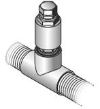
The Waterspace bath drain is to be connected to the sewage system in the room. We recommend to use a trap to avoid unpleasant smell.
