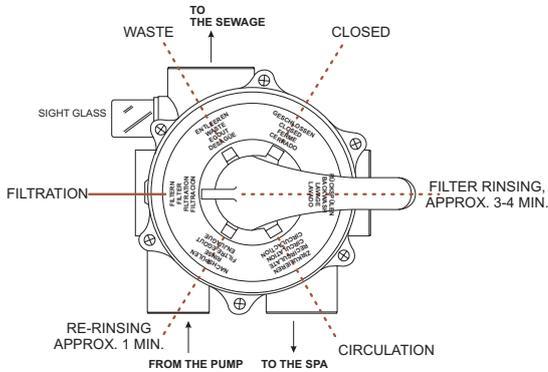
FILTERN, FILTER, FILTRATION, FILTRACION - filtration (regular operation)
