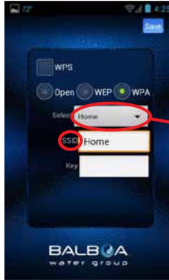
On the Wi-Fi screen you can use the drop down menu to select your network SSID or you can enter it in the SSID box. You will also need to choose the type of password encryption you are using: Open, WEP, or WPA.
